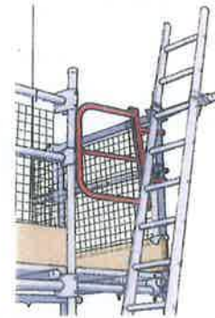
Access ladders should extend 1m above the landing point to provide a strong handhold.
