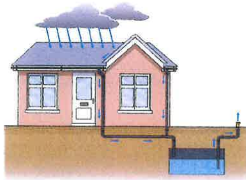
Rainwater gutter flowing down pipes and into drain
